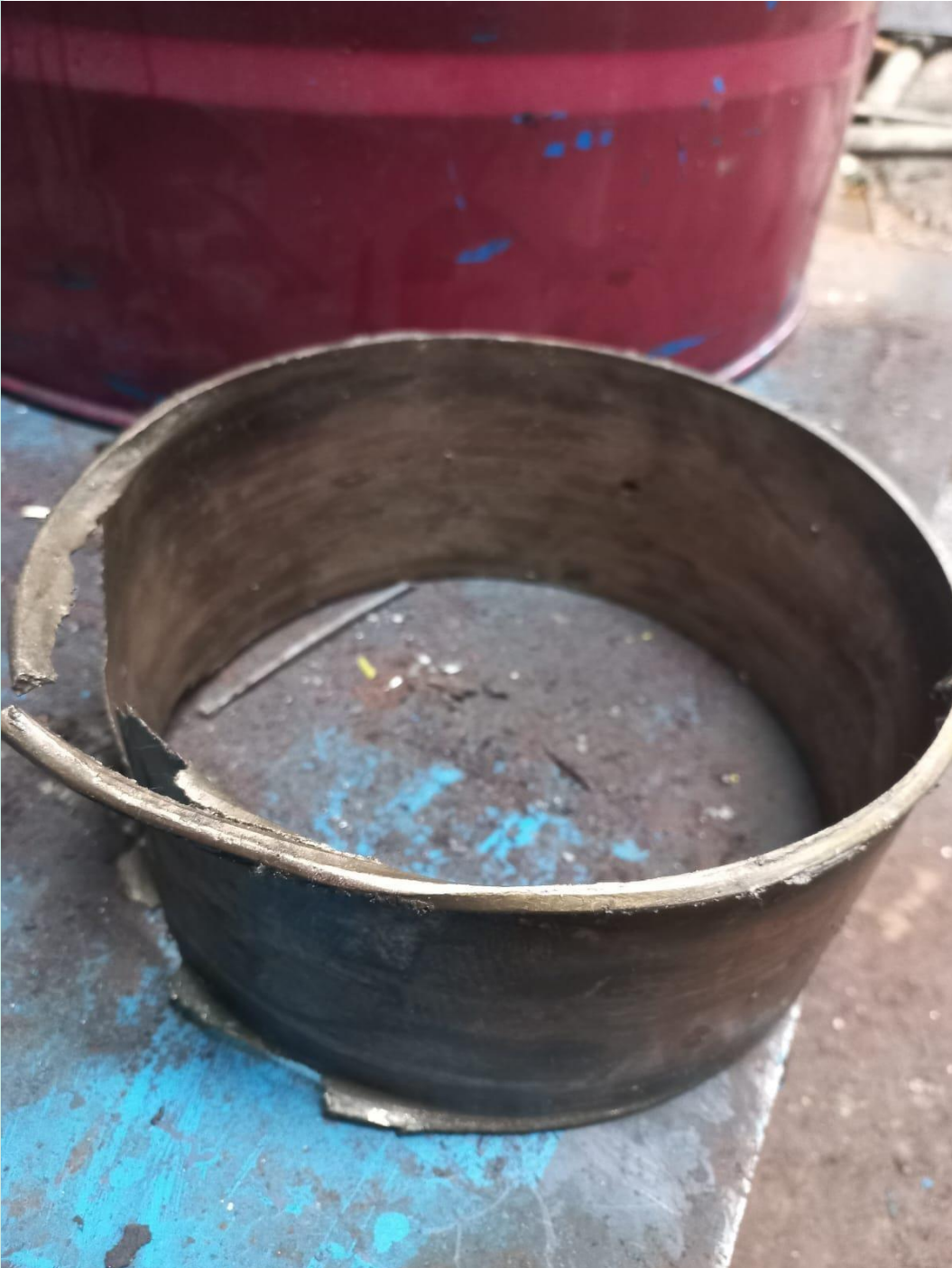
Lampiran 1 Bukti Kerusakan Bushing Crankshaft
