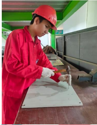
Lampiran 1 Proses Menitik Base Plate Panel
