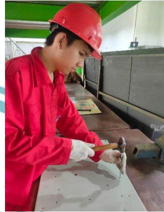
Lampiran 2 Penitikan Base Plate Panel
