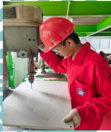
Lampiran 4 Proses Bor Base Plate Panel
