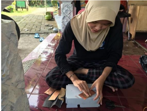
Proses Pengamplasan PCB
