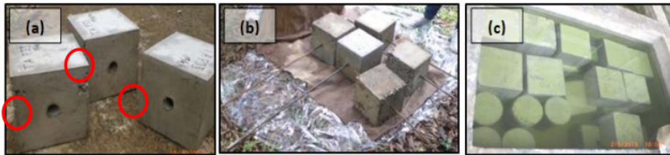
Fig. 2. Specimens in laboratory: (a) hole for steel bar and grouting; (b) monolith concrete; and (c) curing process
